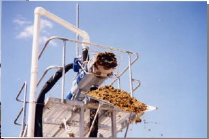
Stand - allows for a pile to be built in front of the separator assisting handling and composting
