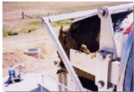
Solids outlet - easy adjustment allows for solids to be drier or wetter depending on preference.
