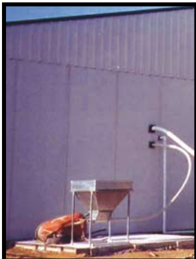
Outside Hopper (80 kg capacity) with minerals auger line to platform dispenser
